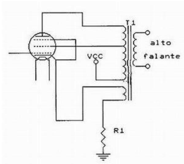
**Fig. 2 - LM3 Output Stage**
