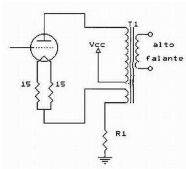
**Fig. 1 - Triode with Partial Cathode Coupling**
